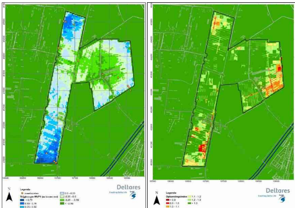
Figure 3. Left: The modeled hydraulic head in the upper aquifer, referenced to ground level. At the edges of the polder, the hydraulic head rises up to 80 cm above ground level causing high risk for boil development. Right: The risk for the development of saline boils for the MT-polder. A value lower than 1.1 indicates a high risk for boil development, a value higher than 1.1 indicates a low risk.
