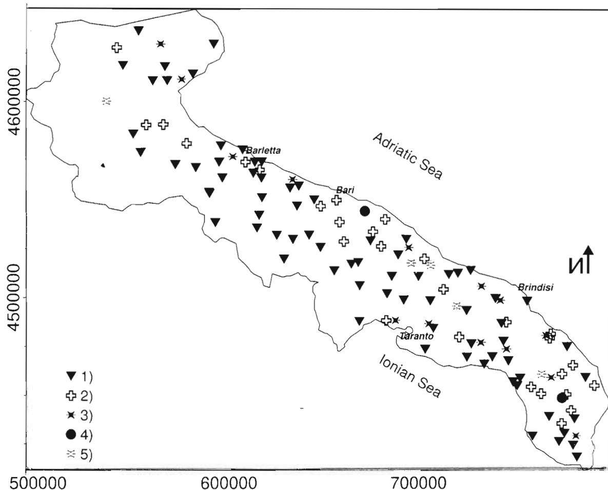
Figure 2. Apulian hydrogeological monitoring network. 1) Piezometric wells, 2) Quality control wells, 3) Sea-water intrusion observation wells, 4) Wells of type 2 and 3, 5) Radio link.
