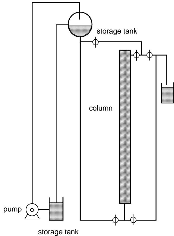
**Figure 1:** Apparatus used for the column experiments.
