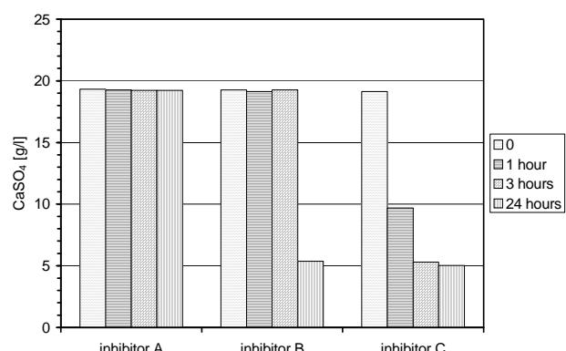
**Figure 4:** Stability of gypsum forming solutions prepared by mixing of Ca(OH)<sub>2</sub> and diluted sulphuric acid.
