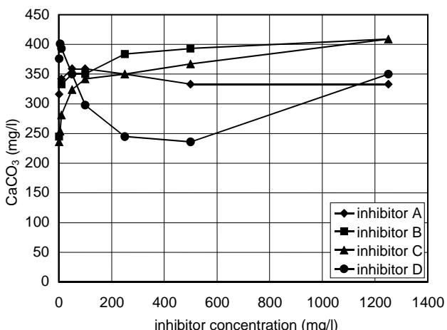
**Figure 5:** Stability of CaCO<sub>3</sub> oversaturated solutions depending on the used inhibitor and its concentration.
