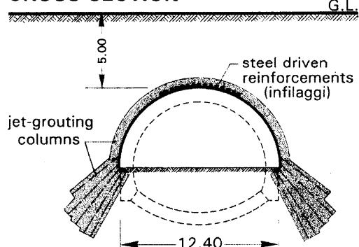
Figure 21: Turin railway junction. Soil improvement for a tunnel (standard section).
