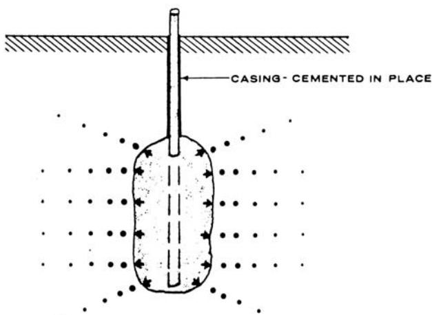
**Figure 13:** Increasing mass of grout displacement and compacting soil as it grows underinjection pressure (After Warner 1982).
