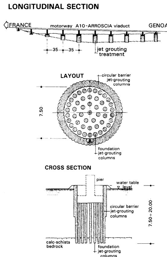
Figure 20: Motorway A10 from Genoa to France (Italy). Arroscia viaduct foundation.
