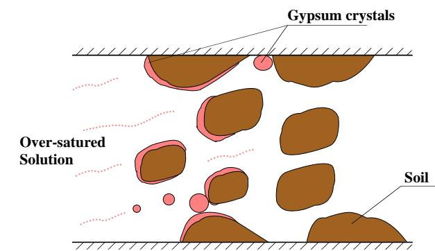
**Figure 2:** Definition diagram of the crystallization process.
