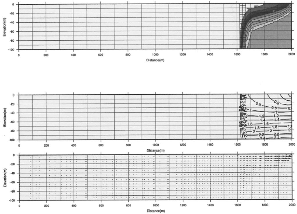
**Figure 7:** Salt concentration, reference head and flow field, Case c5.
