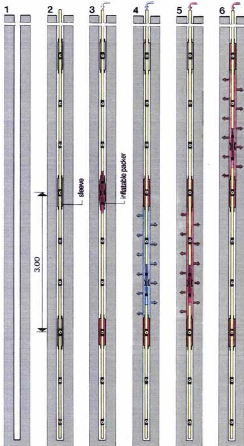
**Figure 6:** M.P.S.P. grouting system (Multiple Packer Sleeved Pipe).
