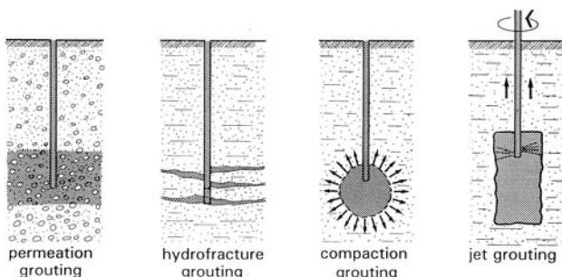
Figure 1: Typical grouting techniques.
