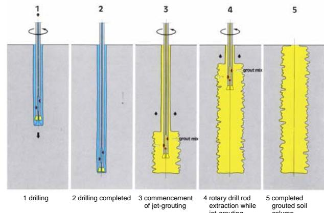
**Figure 15:** Single fluid system working phases.
