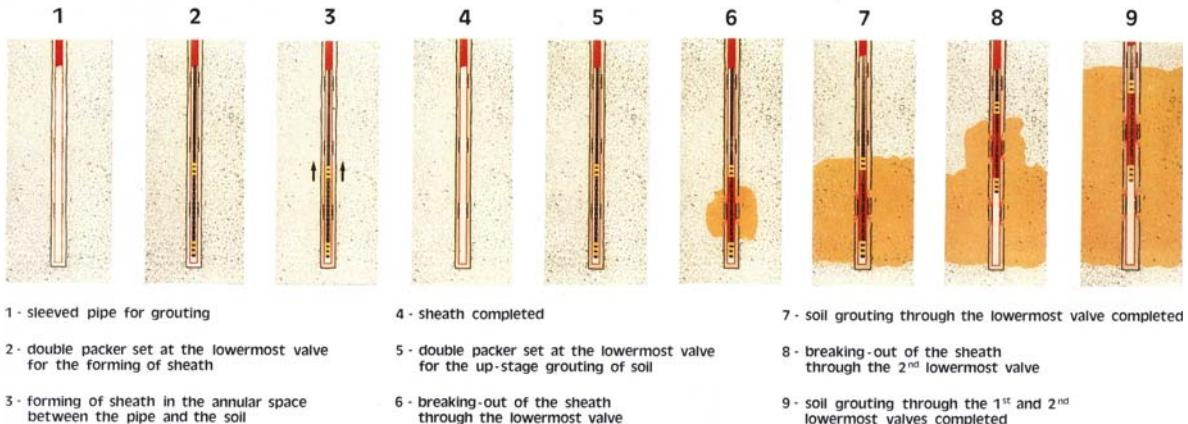
**Figure 5:** Up-stage method by sleeved pipe system.
