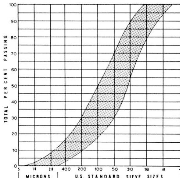
**Figure 14:** Preferred Gradation of Sand Material (After Warner 1982).
