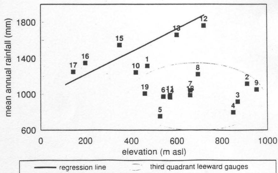
Figure 3 Long duration gauge elevation plotted against rainfall
